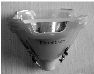
图 1 超高压水银投影灯泡 Fig. 1 Ultra-high pressure mercury lamp
